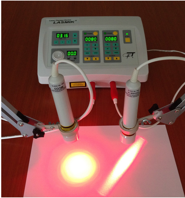
Fig. 2 - The light spot of two sources with one wavelength (635nm): LED bottom left (power 60 mW) and laser diode-bottom right. (power 15 mW)
